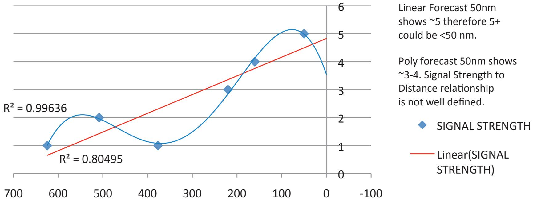
Figure 11 – Radio Signal Strength versus Distance Plot.
