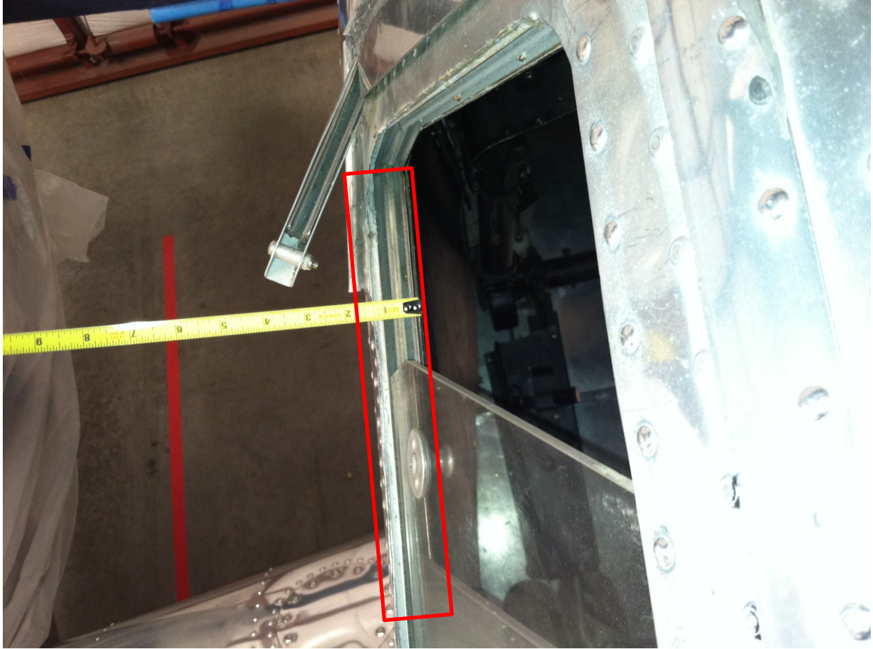
Figure 4: Top-down view of the window slide rail is indicated. This is the rail in which the window travels.
