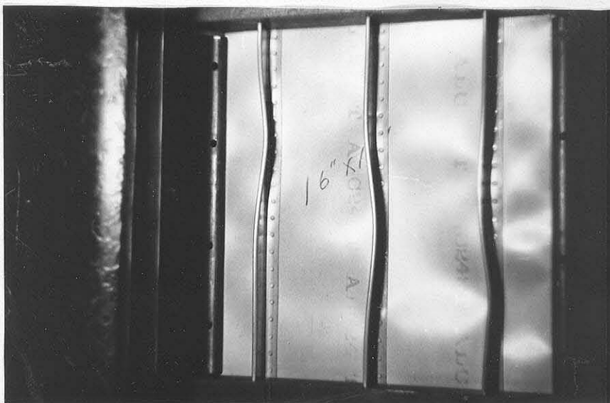
FIG VII TEST PANEL FAILED
