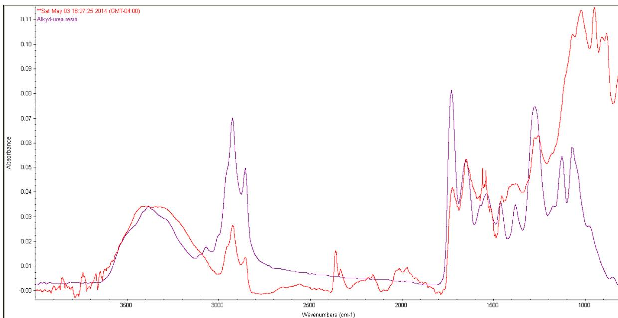
Note that in both samples the aircraft paint fragment reveals that the paint binder is an alkyd resin. Alkyd resins are synthetic drying oils that were invented in 1901, patented by General Electric in 1914, and commercialized by GE in 1926 (see MFA Boston, CAMEO database, Encyclopedia of artists' materials, Alkyd resins). There appears to be a second component of the paint with peaks below 1000 cm-1. This may correspond to aluminum hydroxides formed in the paint over time.
