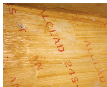
Example of undated ALCOA labeling identical to that on 2-2-V-1. The yellow zinc-chromate wash must have been applied after 1939.
