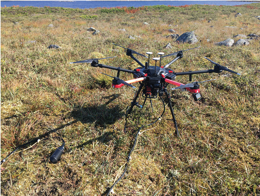
Six-rotor drone operated by Pioneer Explorations. The magnetic sensor was at the end of a five meter tether flown five meters above the water surface in transects five meters apart.
