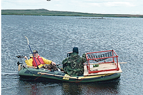
TIGHAR members David Scott (L) and Kenton Spading operated an EM61 mounted on an inflatable boat powered by an electric trolling motor. TIGHAR photo by R. Gillespie.
