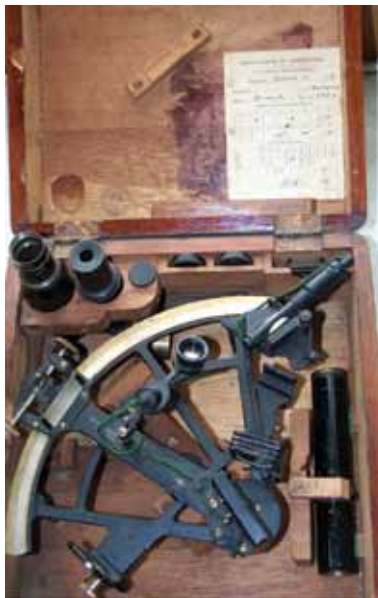
"Byrd" sextant. Brandis Navy Surveying Sextant with bubble modification for aeronautical use.
