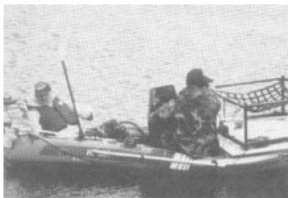
Dave Scott, L, and Kent Spading use the Geonics EM61 to search the pond for metal hits. TIGHAR photo by R. Gillespie.
