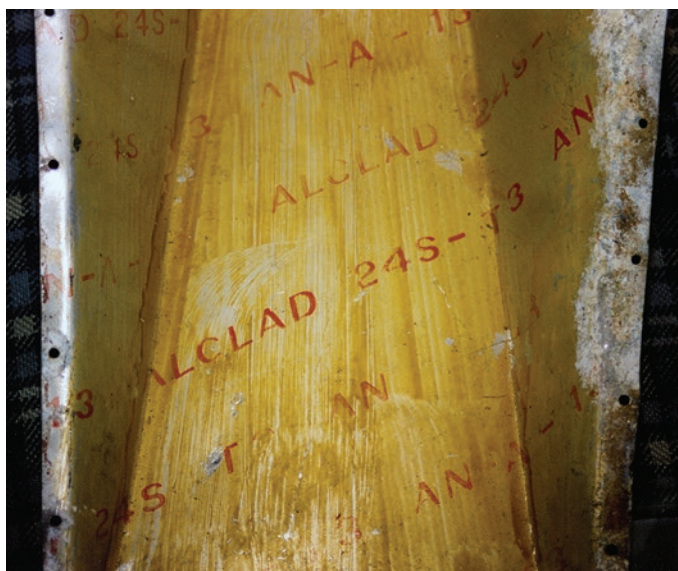
The style of the labeling on 2-2-V-1 is similar to, but not exactly like, the labeling on this flap actuator cover from Electra cn1052 delivered in February 1936. The "AN-A-13" specification included in the labeling seems to date from between 1941 and 1943, so the cover must be a replacement.
