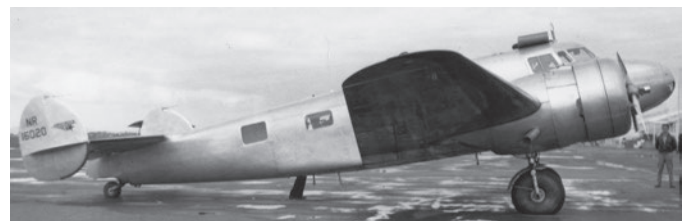
March 1937. The large window installed on the starboard side of the aircraft was in the lavatory compartment at the rear of the cabin. TIGHAR collection.
