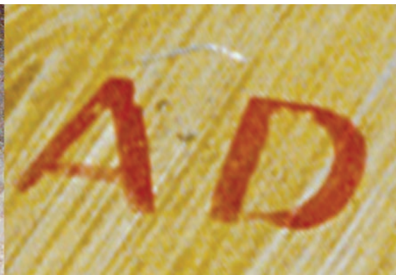
The style of the labeling on 2-2-V-1 is similar to, but not exactly like, the labeling on this flap actuator cover from Electra cn1052 delivered in February 1936. The "AN-A-13" specification included in the labeling seems to date from between 1941 and 1943, so the cover must be a replacement.
