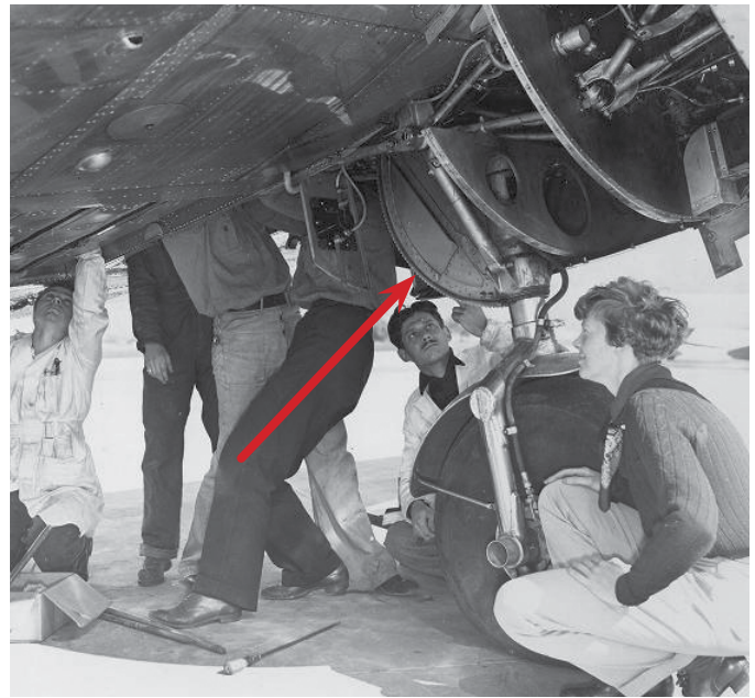
In this photograph the worm gear can be seen on the left main landing gear strut of Earhart's Electra.
