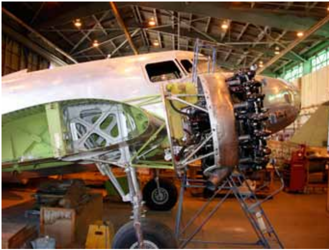
In this photo of Lockheed Model 10A c/n 1130, under rebuild at the National Museum of Naval Aviation, the "new" retraction system – Installation 45100 – is clearly visible.
