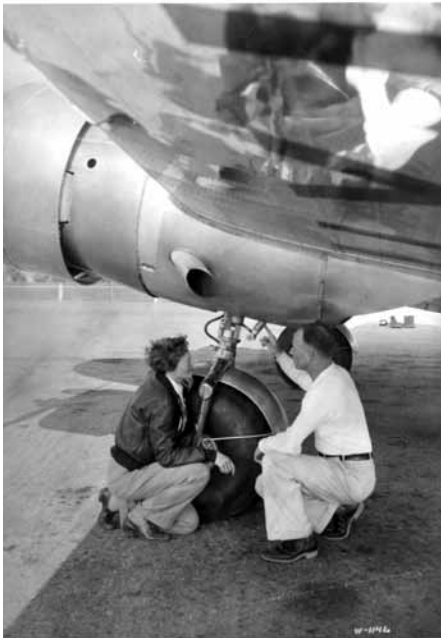
In this photo of Lockheed Model 10A c/n 1130, under rebuild at the National Museum of Naval Aviation, the "new" retraction system – Installation 45100 – is clearly visible.
