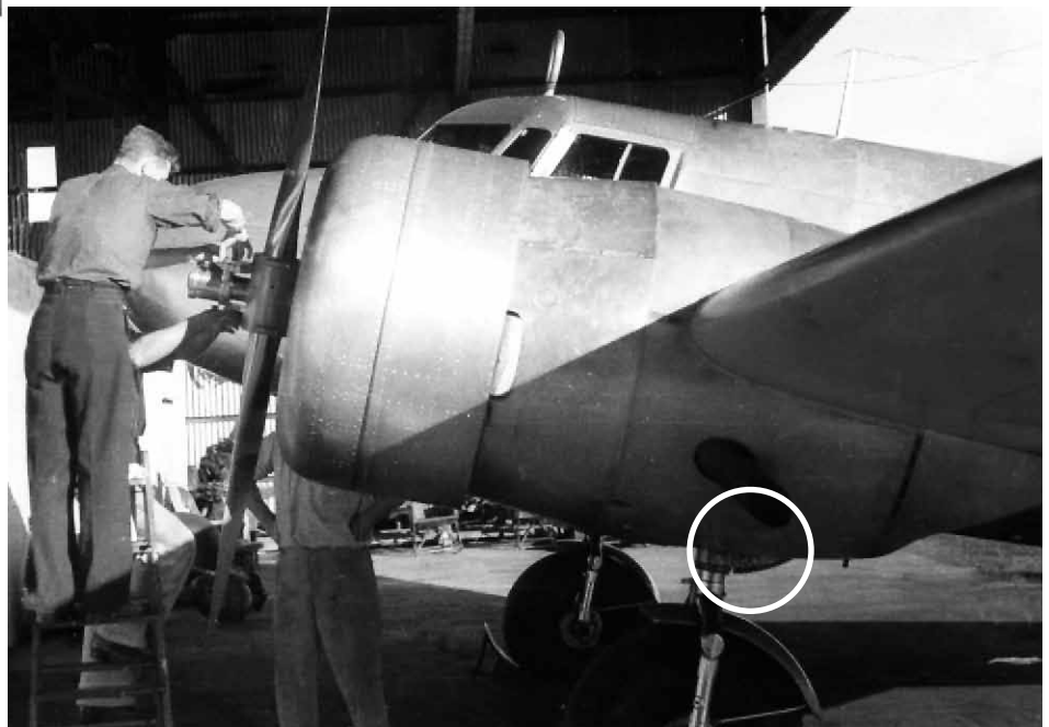
In Lae, New Guinea Fred Noonan assists with maintenance on the left engine propeller hub of NR16020. The bottom edge of the worm gear is clearly visible on the rear side of the left main landing gear strut.
