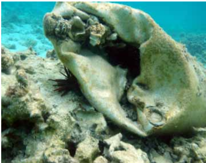
The aluminum skin of the Buffalo's tail cone appears free of any significant coral growth or corrosion. NOAA/Cathy Green.
