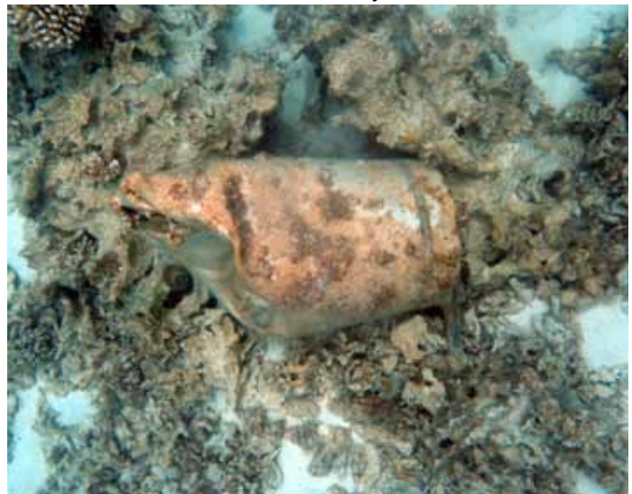
The tail cone was apparently torn loose as the aircraft flipped inverted. The tail wheel was found at the opposite end of the debris field. NOAA/Cathy Green.
