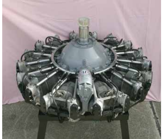
The Buffalo's Wright R-1820-40 Cyclone, was similar in construction to the Electra's smaller Pratt & Whitney R-1340 S3H1 Wasp engines.
