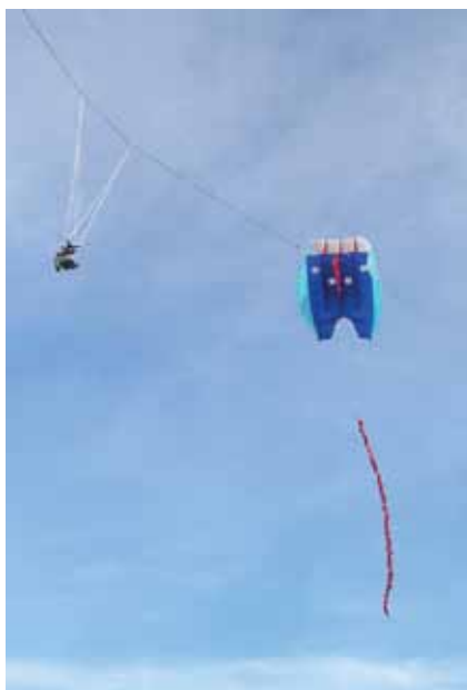
Kite Aerial Photography (KAP) uses a small digital camera mounted in a powered cradle suspended from the string of a kite flown over the target area. It's an economical way to get high-resolution aerial photos in remote locations. Pole Aerial Photography (PAP) uses the same principle but the camera cradle is attached to a long pole. TIGHAR photo.
