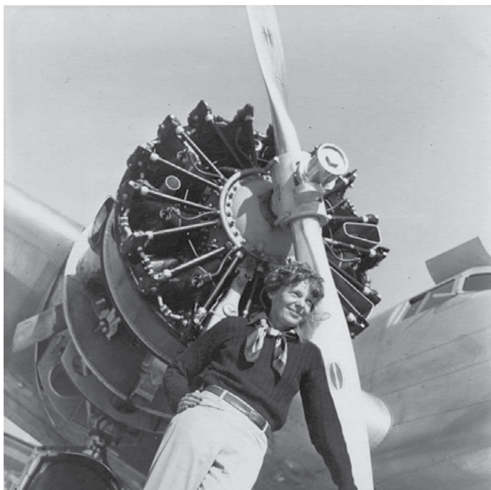
The two 550 hp Pratt & Whitney R-1340 S3H-1 "Wasp" engines weighed 805 pounds each.
