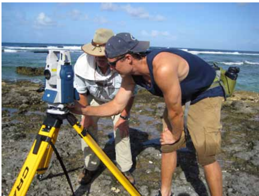
Ric and Josh Gillespie use the Sokkia SRX Robotic Total Station to survey the reef during Niku V. TIGHAR photo by Robin Acker.
