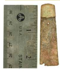
**Artifact 2-8-S-5** is the broken brass liner and nickel-silver bolster from a bone handled, double-bladed "Easy Open Jack Knife" manufactured by The Imperial Cutlery Company of Providence, RI. some time between 1930 and 1945.
