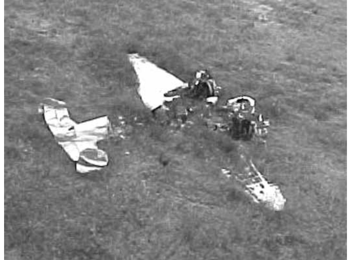
Because the fuel is in the inboard wing sections, post-crash fires often destroyed the cabin area. This is all that is left of c/n 1005 after it nosed over while making an off-airport landing in northern Canada.
