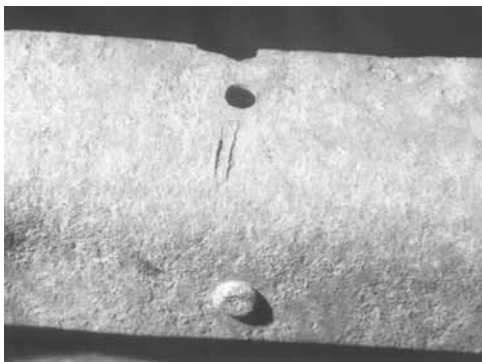
Apparent pry marks on bottom of right angle flange. TIGHAR photo by F. Lombardo
