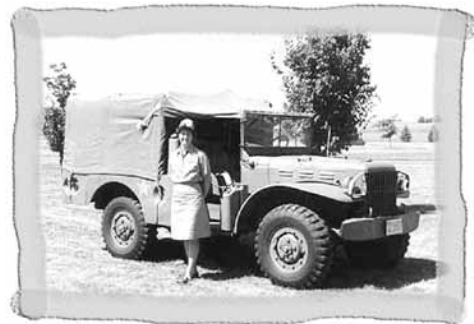
The U.S. Coast Guard Loran station that was located at the southeast end of the island from 1944 to 1946 had a four-wheel drive pick-up truck type of vehicle known as a Dodge WC51 Weapons Carrier. Photo courtesy RobertsArmory.com
