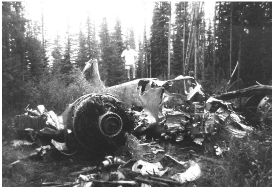
In this photo, taken a year before, the fuselage was still intact. Compare with previous photos, in which large sections have been cut out, including the cabin door, gunner's windows, a substantial portion of the belly and a complete bulkhead assembly, thus destroying the structural integrity of the fuselage. Photo courtesy Bill Carter, TIGHAR #2313CE.
