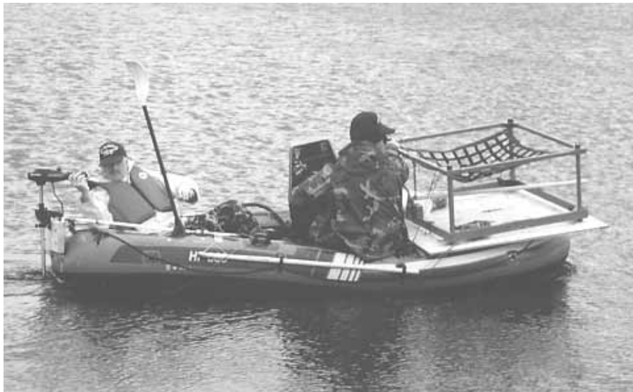
TIGHAR pioneered the use of water-borne electromagnetic (EM) sensing in aviation archaeological applications during field operations in Newfoundland. Here Dr. David Scott and Kenton Spading use a Geonics EM61 to search for the remains of the lost 1927 aircraft l'Oiseau Blanc. TIGHAR photo by R. Gillespie.
