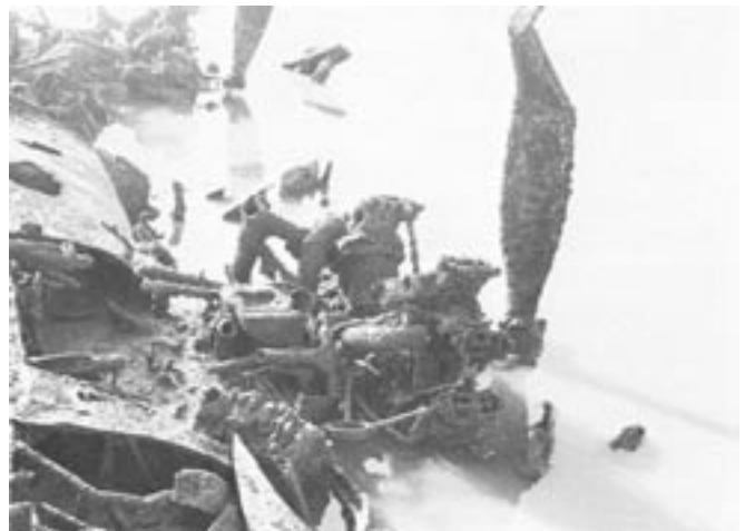
The two 775 HP Wright R-1820-25 Cyclones lie where they came to rest 55 years ago.
