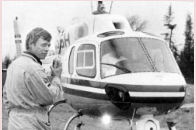
Search leader Ric Gillespie and the Aerospatiale Twinstar. The forward looking infra-red turret is visible under the nose.
