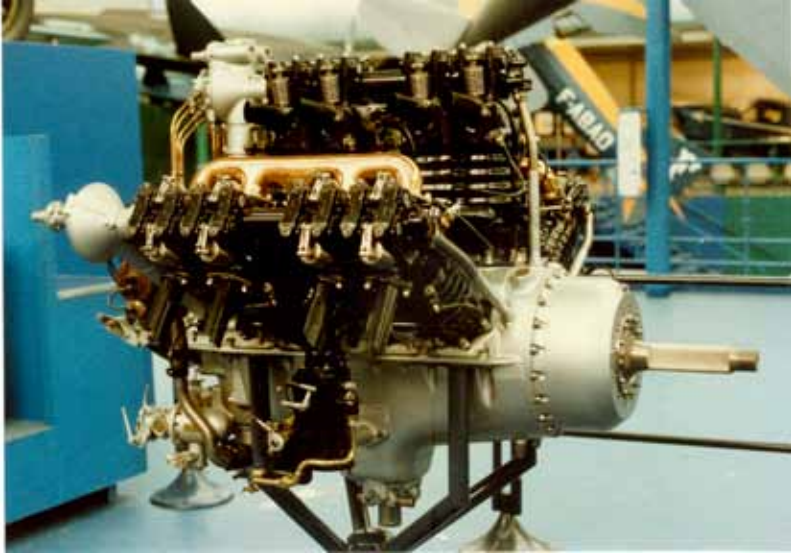
L'Oiseau Blanc was powered by a 450 hp 12-cylinder Lorraine Dietrich engine like this one on display at the Musée de l'Air. TIGHAR collection.
