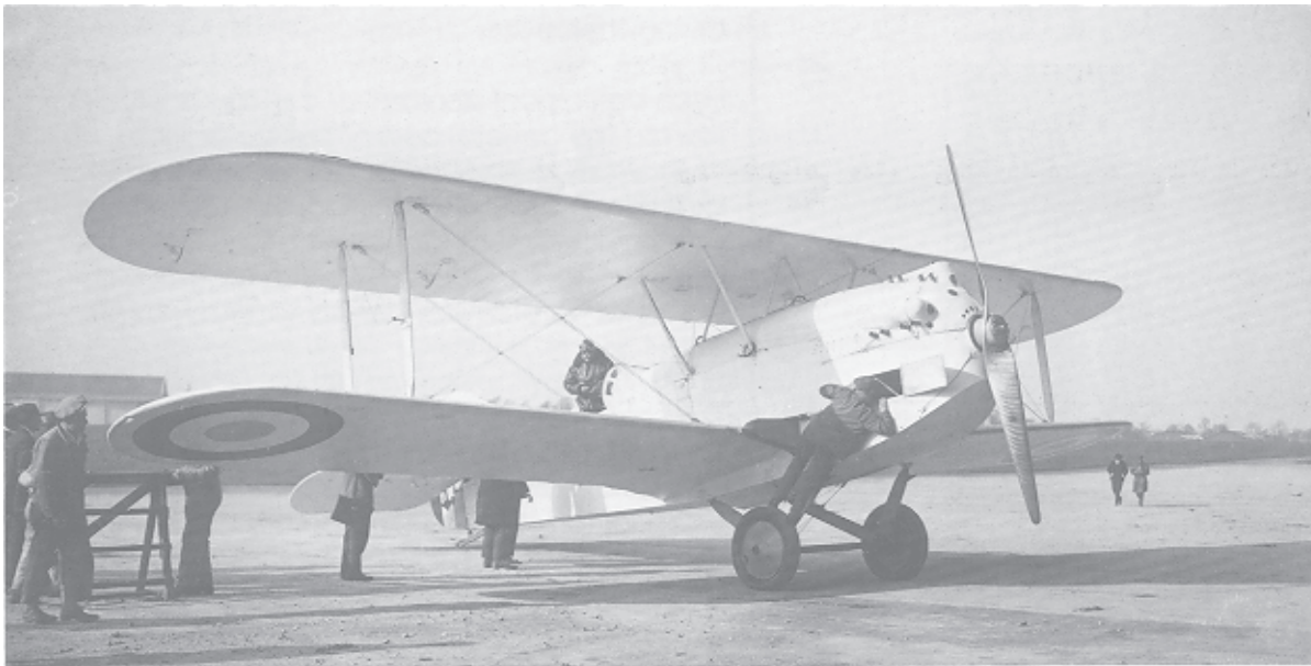
L'Oiseau Blanc during early tests (no nav lights yet). Coli stands in the cockpit. The hatch in the nose provides access to the manual primer for starting. Photo courtesy Musée de l'Air.
